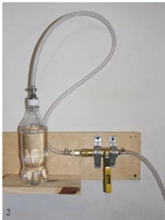
By using a different quick-connect hose the system can be used to carbonate liquids in regular commercial soda bottles.
