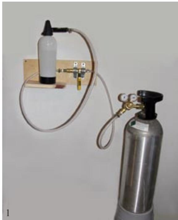
The complete soda making system with a rechargeable siphon bottle.
