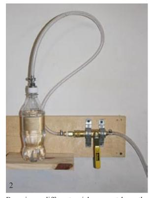
By using a different quick-connect hose the system can be used to carbonate liquids in regular commercial soda bottles.
